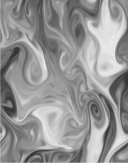
Figure 5.21 Computer simulation of a passive scalar in isotropic turbulence at a Schmidt number of 25. (Picture by G. Brethouwer and F. Nieuwstadt, University of Delft. Courtesy of efluids.com.)
